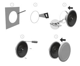
**Note:** when making the hole in your mounting panel, double check if there are no cables or any other obstructions behind the mounting panel. Cutting the mounting panel without this check might result in damaged infrastructure or power lines.
